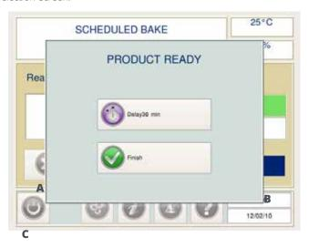
If delay was selected, and the delay cycle is complete, the 'Product Ready' screen will be displayed again. **Please note that the delayed time duration will be displayed on screen.** Press 'OK' to acknowledge the end of the cycle. The retarder prover will resume a retard cycle whilst displaying the 'Program Selection' window.
